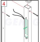
Put in the lock, pull out the power lines.
